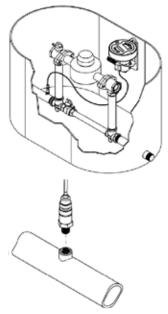
2 Apply joint-sealant and thread pressure sensor into 1/4" NPT port. Turn on the water.
