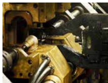
Stem is electrically heated and thrust together to create the thrust collar
