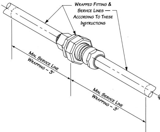
**CAUTION:** Read and follow these instructions to install the Mueller® Insulated Straight Service Fitting. Failure to do so may result in damage to the fitting and/or piping system, or may prevent the insulator from functioning as intended.
